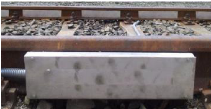
Picture 1: Flat detection system, assembled at track
